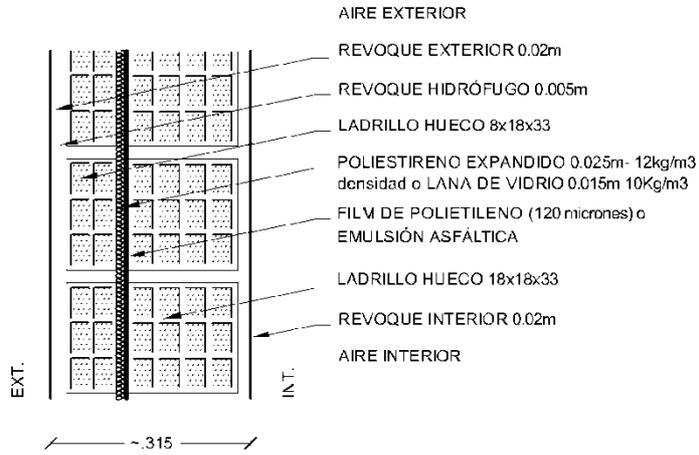
MURO DOBLE LADRILLO HUECO DE 8/ HUECO DE 18 + AISLACION (7CAPAS) K=0.60 W/m<sup>2</sup>K
