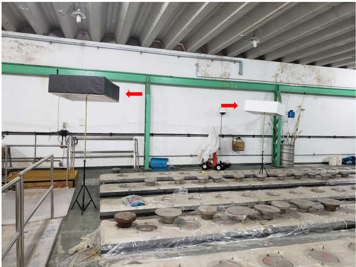
Figure 4– White and black boxes used to test the response of the LCCT
