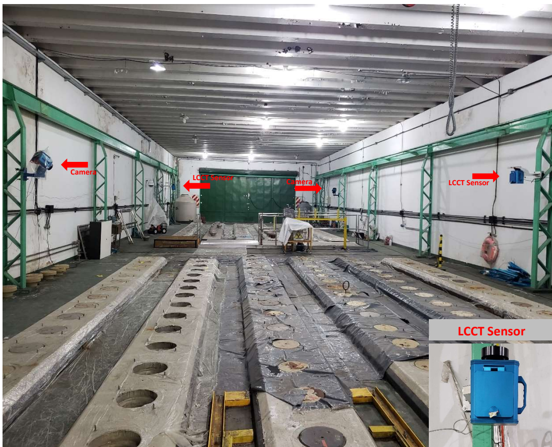
Figure 2– Perimeter acquisition and ROI setup
