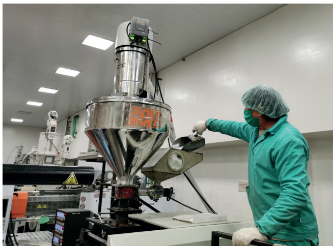
Carga manual de pellets (materia prima y masterbatch).
