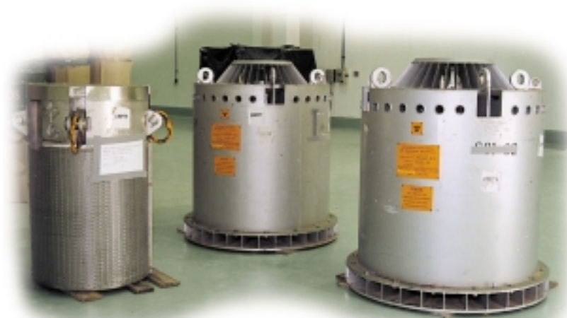
Type B (U) packages for cobalt 60 transport, referred to as GURI 01
