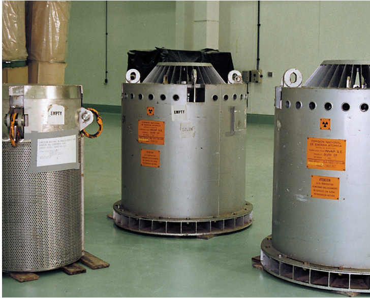
Type B (U) packages for cobalt 60 transport. GURI 01 (centre and right) and F129 (left) models.
